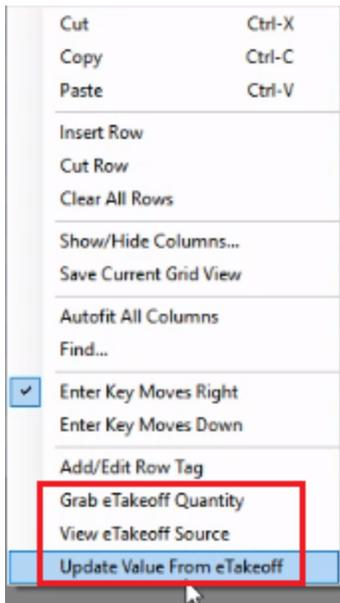
**Grab eTakeoff Quantity** is one of three eTakeoff-related options that appear on the shortcut menu. If you right-click a quantity that originated in eTakeoff, the **View eTakeoff Source** and **Update Value From eTakeoff** options are available.
